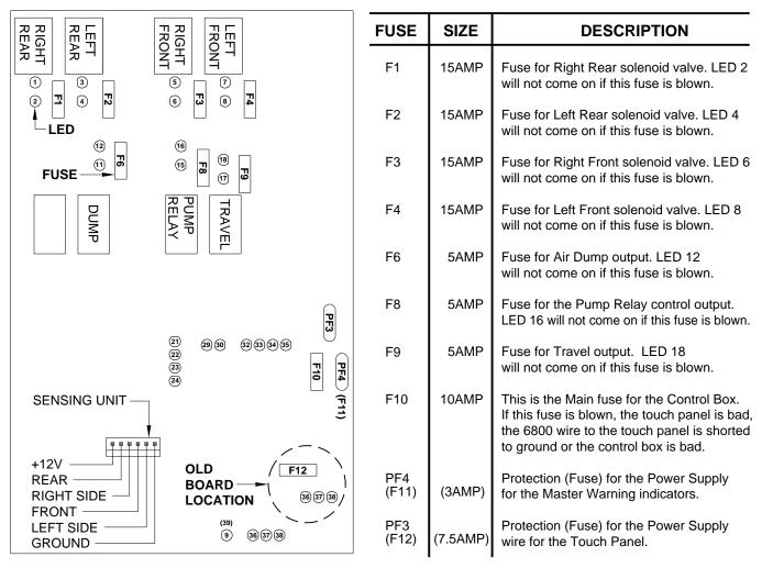
NOTE: On newer control boxes, FUSE F11 and FUSE F12 have been replaced with POLY SWITCHES PF4 and PF3. Poly switches protect a component or wire as a fuse does except the poly switch will allow current through when the overload or short is removed. Poly switches are not replaceable.
